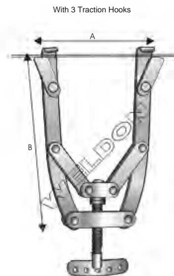
Kirschner WS-256-057 0-40 mm Small Pattern 18 cm / 7 1/4" WS-256-058 35-200 mm Large Pattern 27 cm / 10 1/2"
